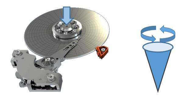
Rotational Vibrations will induce "Precession" of the Spindle Motor, if both ends are not fixed.
